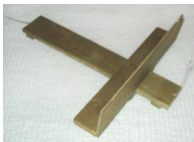
a: Jacob’s stick 2 in Bartoli (1564), I.7 b: instrument constructed by the students
